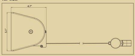
The **Siro** side shade is a multi-functional side shade for privacy, wind control, and low angle sun protection. The lateral shading device is also a great addition to overhead sun protection systems. An integral tension spring component maintains optimum fabric tensioning and the cassette housing provides complete fabric protection when the unit is retracted.
