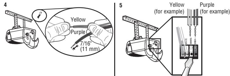
To insert or remove the wires from the terminal, push in the tab with a screwdriver tip.
