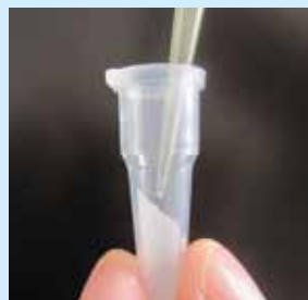
Figure 2 Proper sample application is made directly in to the center of the gel bed.
