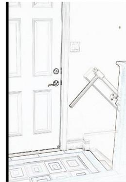
After accommodating any hallways, doors etc. you now must determine the installation height for the user. With the users arms bent at the elbow measure from the floor to the center of the wrist. Use this measurement for the placement of the top of the connection plate. **This is a min.size it can be higher but not shorter.** To find the second measurement for the top of the stairs add 4" to the initial measurement, as seen below.
