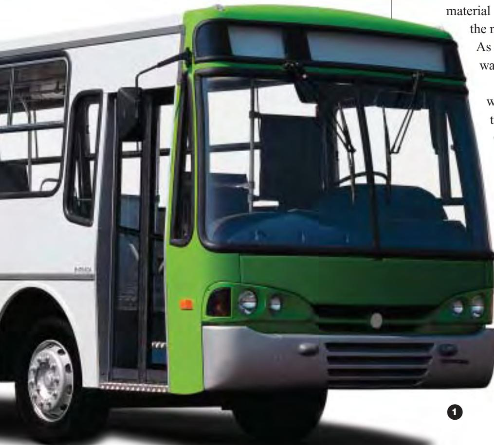
**1** CIFERAL, a bus manufacturer in Brazil, used 3M VHB (very high bond) tape to attach aluminum exterior side panels to the vehicles' frames.
