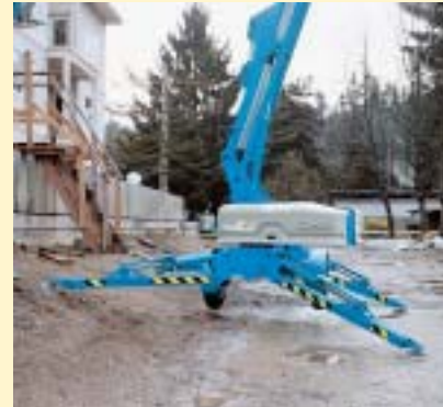
Optional Hydraulic Outriggers with Automatic Leveling System
