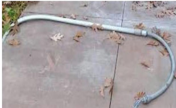
These two pictures are an example of a whip. This is required to be in place on the day of delivery so that we can place the hot tub and attach the whip to the spa in order to test and run it.
