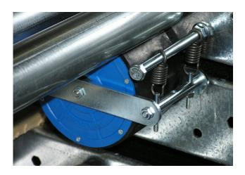
Indirect mount speed controllers are mounted underneath full roller pallet flow systems and are preferred in many cases because they do not make direct contact with the load. Indirect mounting is not recommended for use with steel containers or pallets with steel-bottom runners because of potential skidding of pallet over conveyor rollers.
