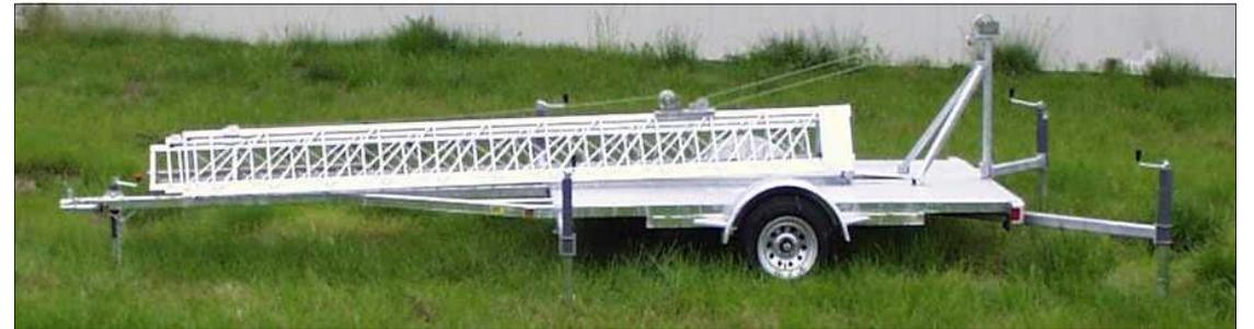
**Figure: 1** Trailer with outriggers fully extended
