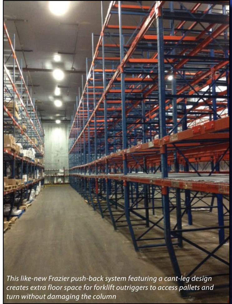
*This like-new Frazier push-back system featuring a cant-leg design creates extra floor space for forklift outriggers to access pallets and turn without damaging the column*
