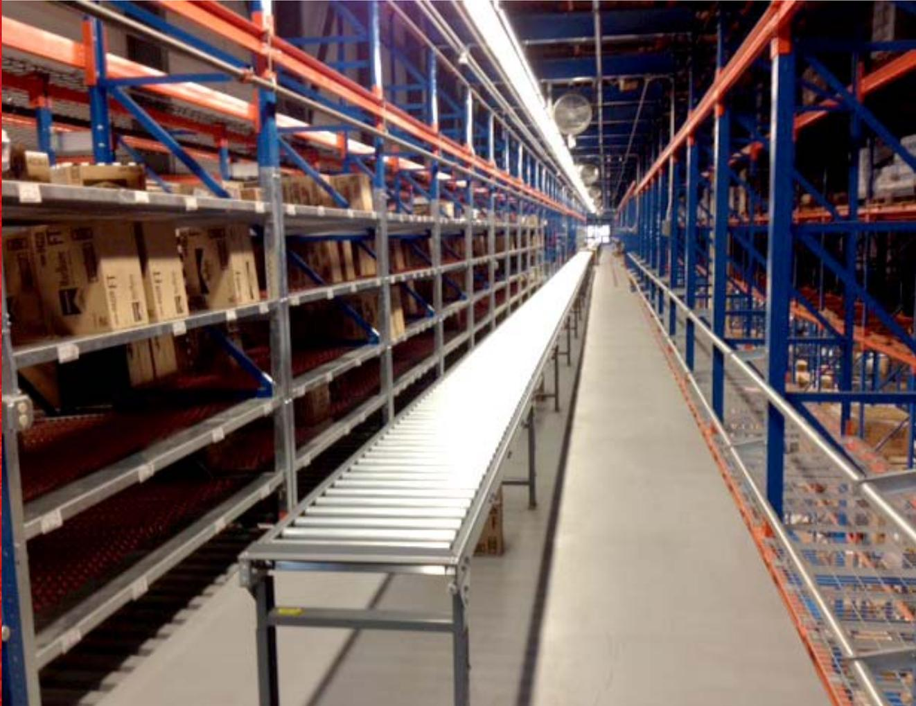
**E-Distribution** case flow systems provide additional selection faces within existing rack bays or pick modules - Up to 5 added shelf levels and approximately 35 pick faces per bay can be created for full case selection or individual item picks from master cartons or trays.
