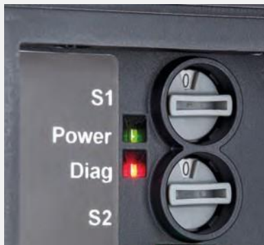
LED indicates status of diagnostics contact
