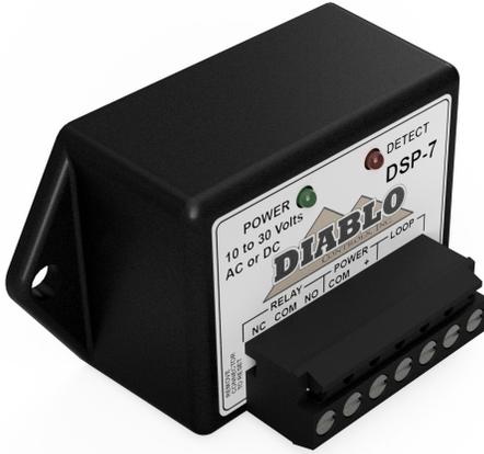
Detector operates on any voltage from 10 to 30 volts AC or DC and draws approximately 35 milliamps of current with no vehicle on the loop. This micro-sized detector has no user settings and will automatically configure itself when powered up. When used with other DSP-6LPs, DSP-7LPs, or DSP-7s, the detector will not cross-talk.
