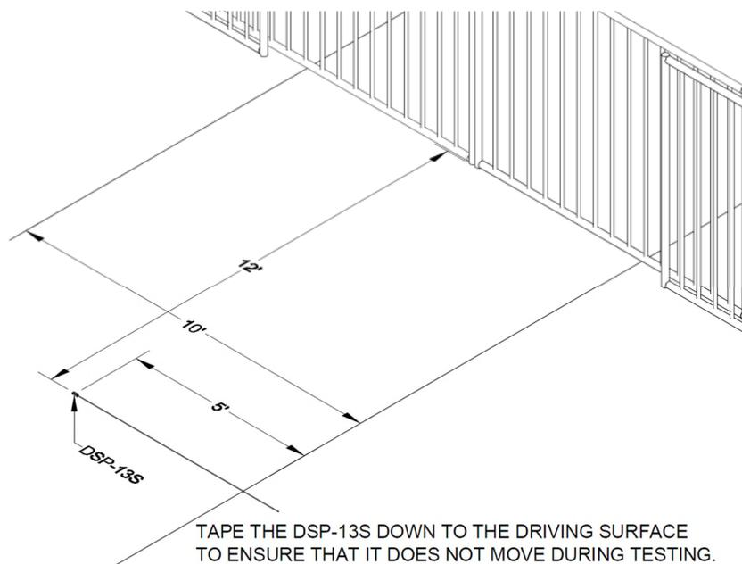
**Figure 7: Sensor Placement**
