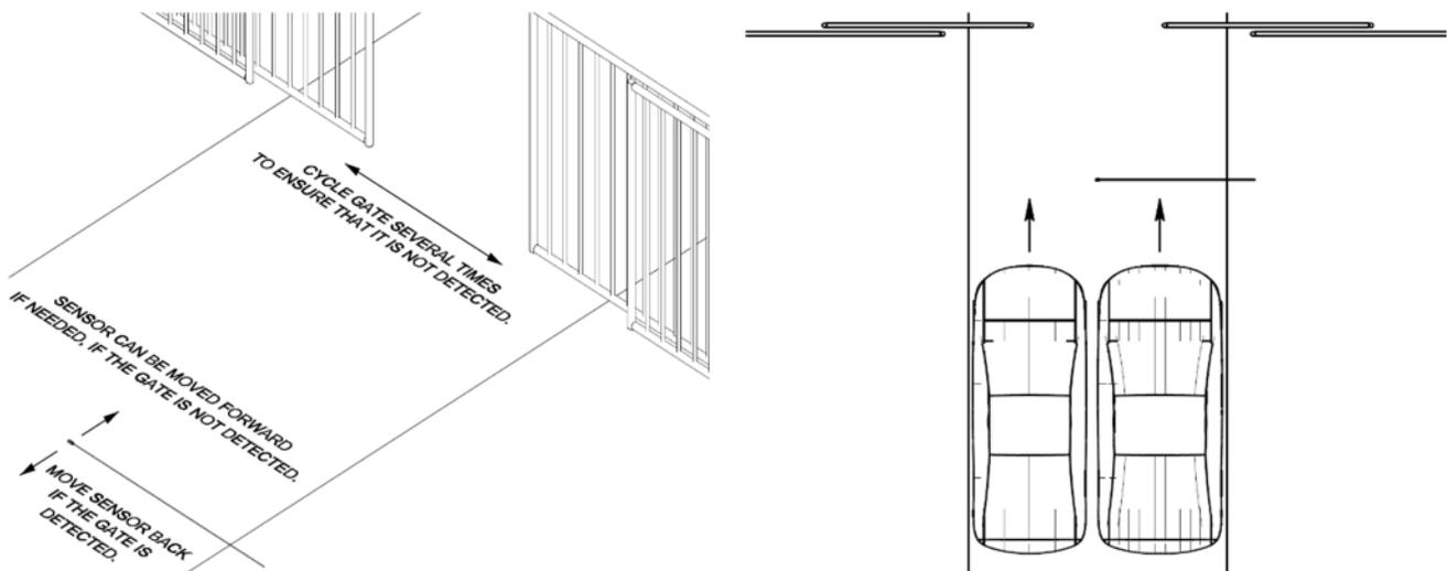
Figure 9: Sensor Placement Testing
