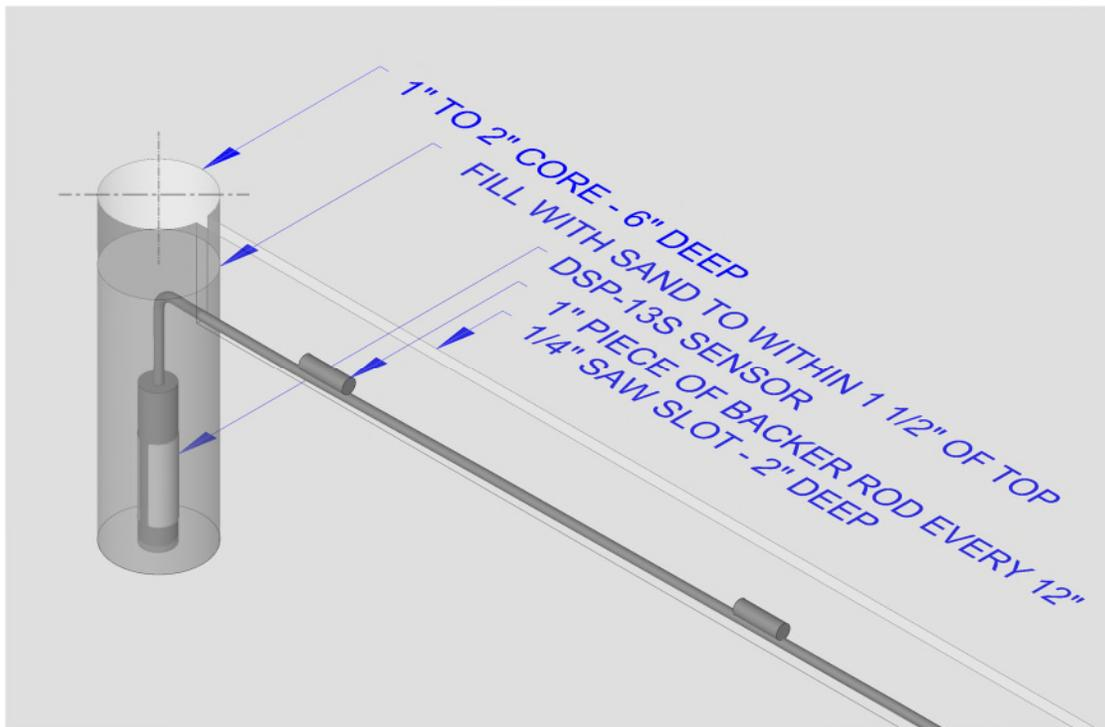
Figure 10: Sensor Installation – Saw Cut & Core
