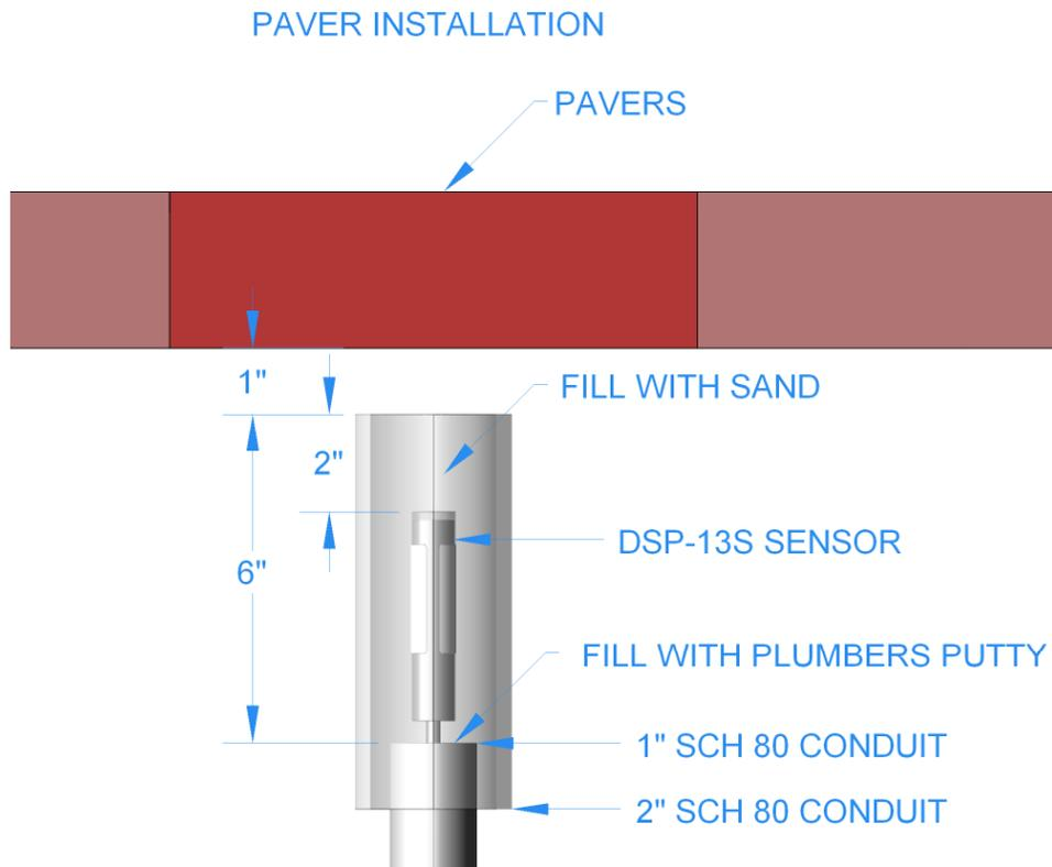
Figure 11: Sensor Installation – Conduit Under Pavers
