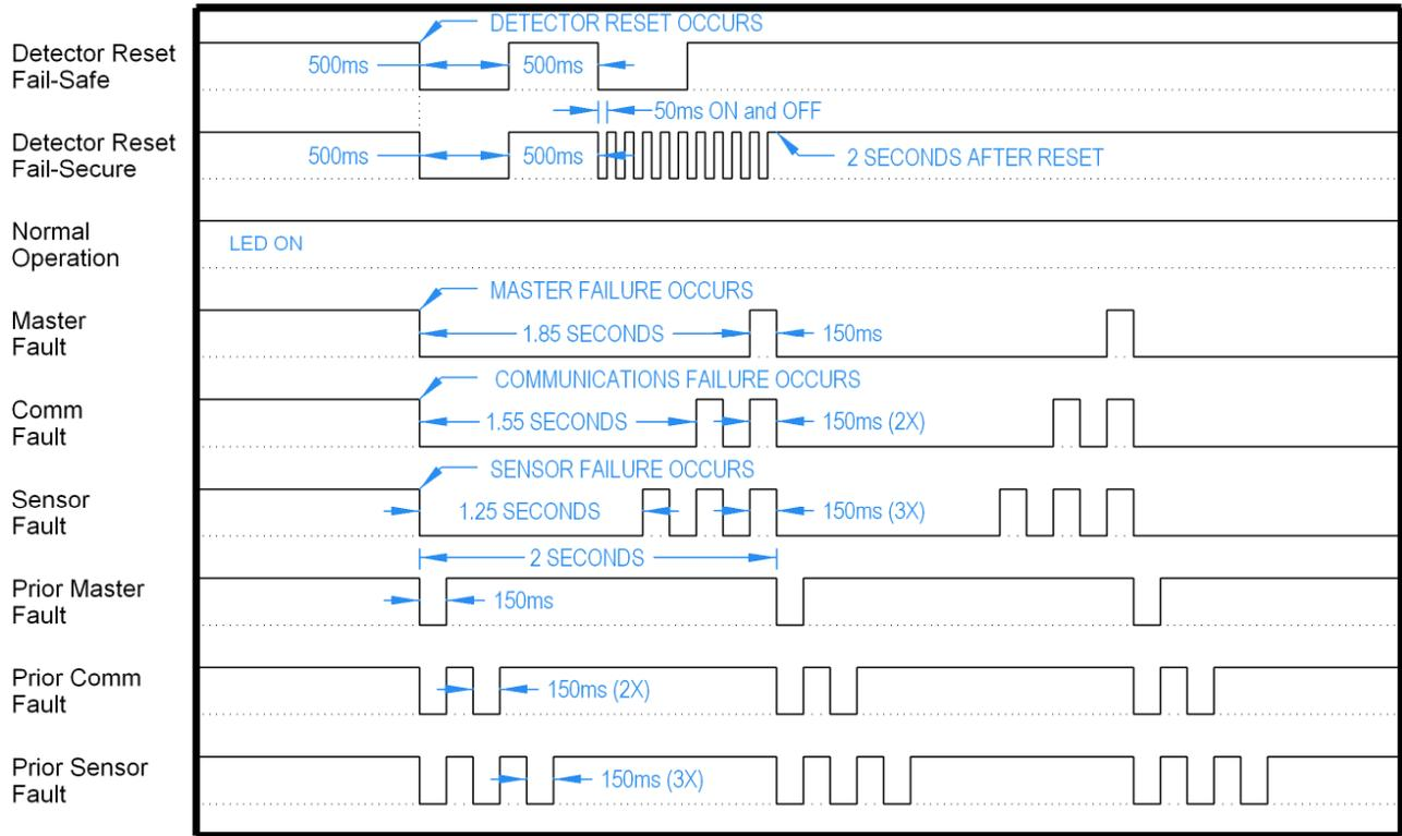
Figure 5: Power LED Displays
