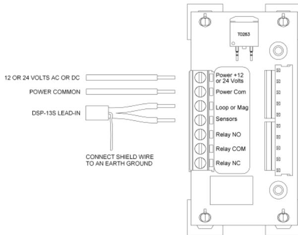
Figure 8: DPS-13 Wiring for Testing
