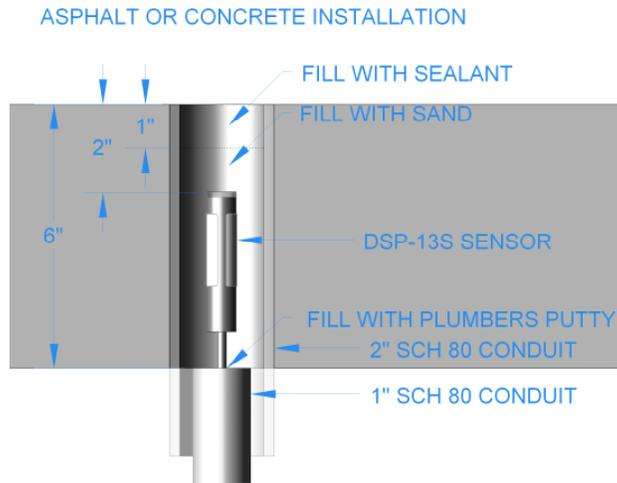
Figure 12: Sensor Installation – Conduit Under Asphalt or Concrete
