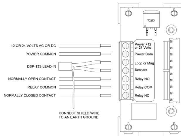
Figure 13: DSP-13 Master Wiring Using an RK1-R
