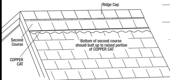
From left, use a roofing flat bar to lift bottom of 2nd course. Slide a COPPER CAT strip under 3/4" to where bottom of shingle butts up to COPPER CAT'S raised portion, nail down, repeat to end.
