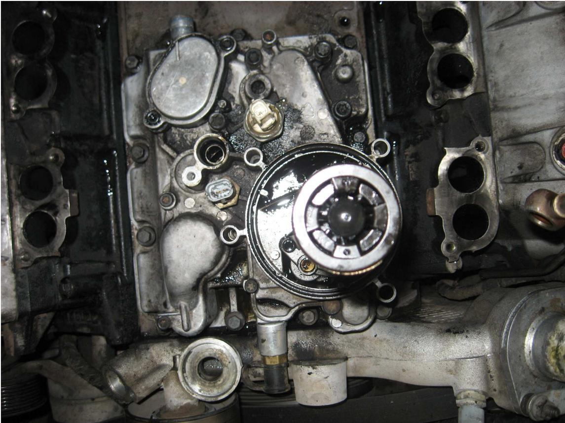
Figure 1 OE Engine Oil Cooler, Top View
